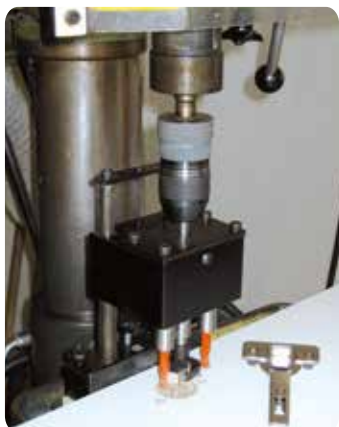
TRIMATIC 48/6 montato su trapano a colonna TRIMATIC 48/6 used with a pillar drilling machine
