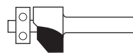
HW FLUSH AND BEVEL TRIM BITS WITH BALL BEARING GUIDE Z=2 Page 1.18
