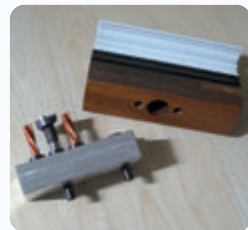
• DRILLING OF WOOD AND PVC • WINDOW FRAME TO • FIT CREMONE BOLT • Page 16.13
